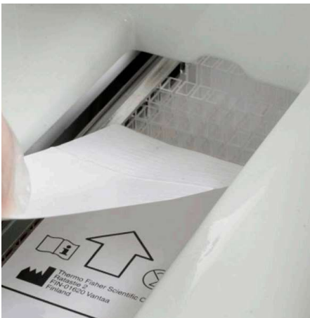
Cuvette loader for 360 cells. Low-volume reaction cuvette uses reagent and water for lower environmental impact.
