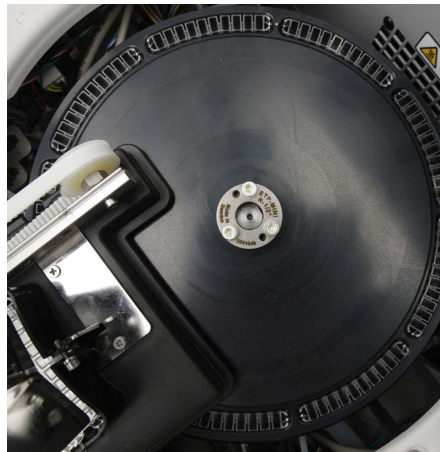
Temperature controlled incubator for 90 cuvette cells. Cuvettes are disposable, so there is no need for extra rinsing to prevent carry-over.
