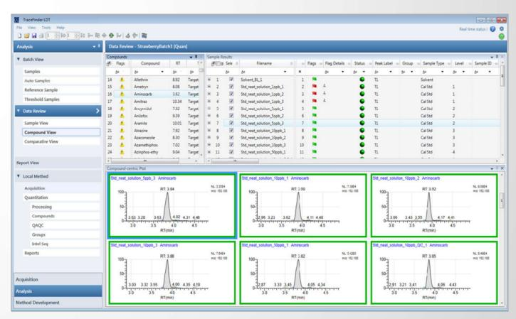
TraceFinder software—provides comprehensive processing methods and improved handling of ion ratio calculations, reviewing, reporting, comparison of mass spectra and data integration.
