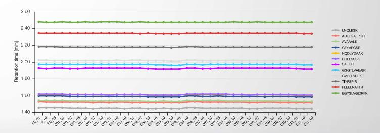
Analytical properties: Variation of detected retention time determined to be less than ±0.01 minutes.
