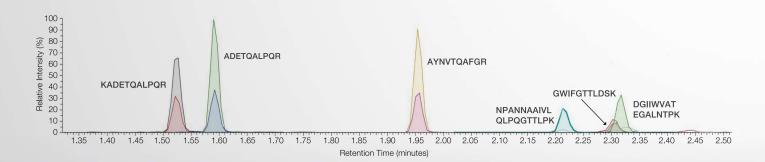
A chromatographic trace demonstrating the separation of the targeted peptides. Each peptide has a less abundant isotope-labeled standard with near identical retention times (±0.01 minutes).
