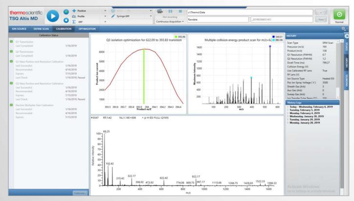
Tune software—calibrate the instrument for maximum performance with a variety of scan types, scan modes, ion polarities, scan rates, and resolution settings.
